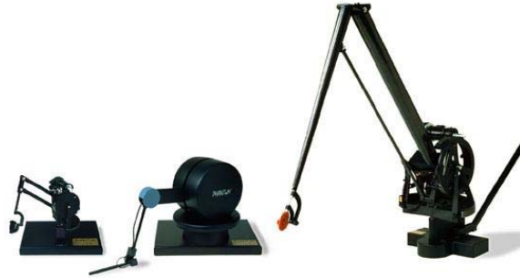
Figure 4.6: Different models of the PHANTOM force-feedback device
